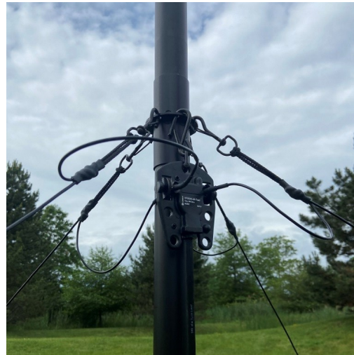
Centre junction and dipole wires (shown with optional AMX85 support mast)
