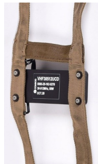
Centre junction of antenna
