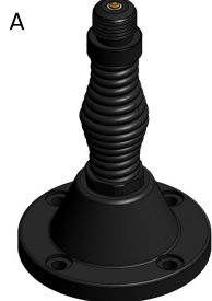
A NATO 4-hole Spring 4 x M10 or 3/8" Bolts on 114 mm PCD Base diameter 140 mm Base height 215 mm
