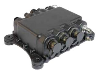
The EZPRR was developed from the basic 256 channel PRR. Data transmission was added to the original voice capability and both voice and data (which can be transmitted simultaneously) are now encrypted. Channel 15 of the EZPRR remains unencrypted to maintain backwards compatibility with the original PRR.
