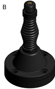
B NATO 4-hole Spring GPS 4 x M10 or 3/8" Bolts on 114 mm PCD Base diameter 140 mm Base height 240 mm
