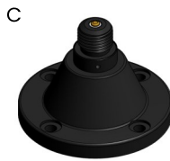
C NATO 4-hole Rigid 4 x M10 or 3/8" Bolts on 114 mm PCD Base diameter 140 mm Base height 100 mm
