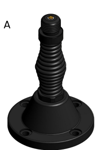
A NATO 4-hole Spring 4 x M10 or 3/8" Bolts on 114 mm PCD Base diameter 140 mm Base height 215 mm
