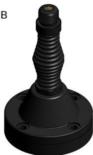
NATO 4-hole Spring GPS 4 x M10 or 3/8" Bolts on 114 mm PCD Base diameter 140 mm Base height 240 mm
