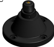
NATO 4-hole Rigid 4 x M10 or 3/8" Bolts on 114 mm PCD Base diameter 140 mm Base height 100 mm
