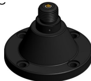
NATO 4-hole Rigid 4 x M10 or 3/8" Bolts on 114 mm PCD Base diameter 140 mm Base height 100 mm
