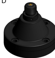
NATO 4-hole Rigid GPS 4 x M10 or 3/8" Bolts on 114 mm PCD Base diameter 140 mm Base height 125 mm
