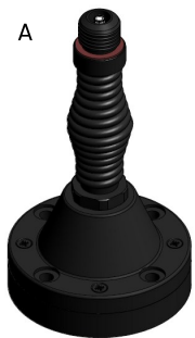
A NATO 4-hole 4 x M10 or 3/8" Bolts on 114 mm PCD Base diameter 140 mm
