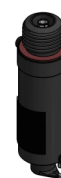
E Tube Clamp Adaptor Clamp area diameter 38 mm Clamp area length 80 mm N-type female bottom connector
