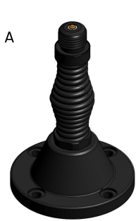
A NATO 4-hole Spring 4 x M10 or 3/8" Bolts on 114 mm PCD Base diameter 140 mm Base height 215 mm
