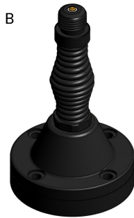
B NATO 4-hole Spring GPS 4 x M10 or 3/8" Bolts on 114 mm PCD Base diameter 140 mm Base height 240 mm
