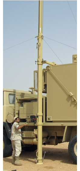
Mast fully deployed
