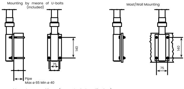
Must withstand moment of flexure (see Mechanical Specifications) Use bolts and nuts M10
