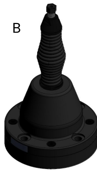
B NATO 4-hole GPS Spring Base 4 x M10 or 3/8" Bolts on 114 mm PCD Base diameter 140 mm Base height 245 mm
