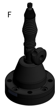
F NATO 4-hole GPS Tilt Spring Base 4 x M10 or 3/8" Bolts on 114 mm PCD Base diameter 140 mm Base height 305 mm
