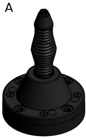
A NATO 4-hole Spring Base 4 x M10 or 3/8" Bolts on 114 mm PCD Base diameter 140 mm Base height 220 mm
