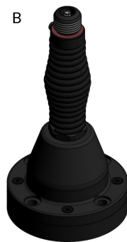
B NATO 4-hole Spring GPS 4 x M10 or 3/8" Bolts on 114 mm PCD Base diameter 140 mm Base height 280 mm
