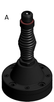
A NATO 4-hole Spring 4 x M10 or 3/8" Bolts on 114 mm PCD Base diameter 140 mm Base height 240 mm
