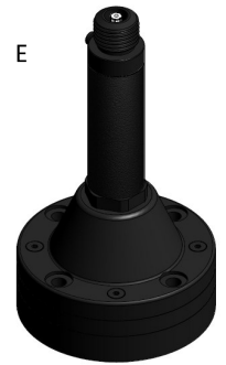
E NATO 4-hole Rigid (no spring) 4 x M10 or 3/8" Bolts on 114 mm PCD Base diameter 140 mm
