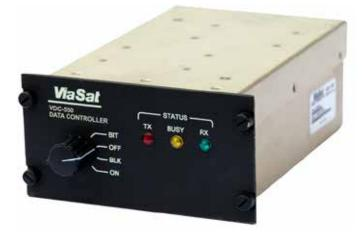
The ViaSat Data Controller 550 (ViaSat VDC-550) enables secure data networking using any combat net radio, linking warfighters on the tactical edge to the Common Operating Picture. Run netcentric web applications, send error-free data, and employ TCP/ IP services over existing radios, even over severely degraded radio channels.
