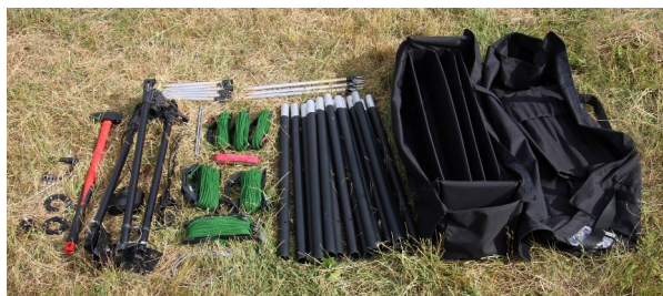
Complete mast kit packs into two man-portable bags (15 m kit)
