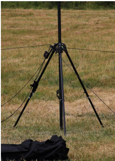
Tripod assembly with mast section hoist and lifting mechanism
