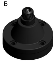
B NATO 4-hole Rigid (no spring) 4 x M10 or 3/8" Bolts on 114 mm PCD Base diameter 140 mm
