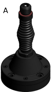
A NATO 4-hole Spring GPS Option 4 x M10 or 3/8" Bolts on 114 mm PCD Base Dia. 140 mm
