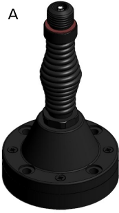
A NATO 4-hole Spring 4 x M10 or 3/8" Bolts on 114mm PCD Base diameter 140 mm Base height 215 mm
