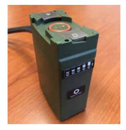
This RPA is the next generation of power management for dismounted soldier systems. The RPA replaces the standard handheld radio battery and connects directly to the Conformal Wearable Battery (CWB), extending mission times. The RPA provides power and data at all times including during the hot swap of the CWB, ensuring the warfighter remains connected to the network for the entire mission.
