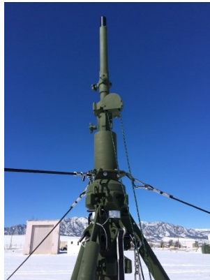
Top load attached to top mast section
