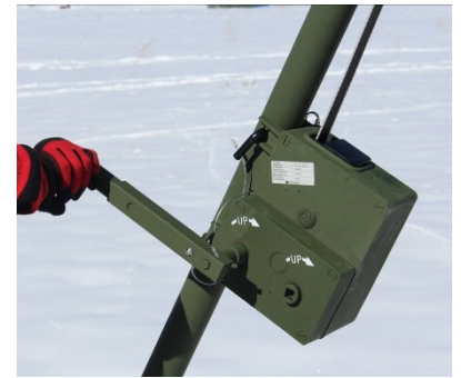
Hand operated lifting winch (motorised version available)
