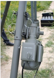
Electric motor for lifting winch
