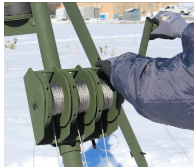
Central guying system maintains tension during deployment
