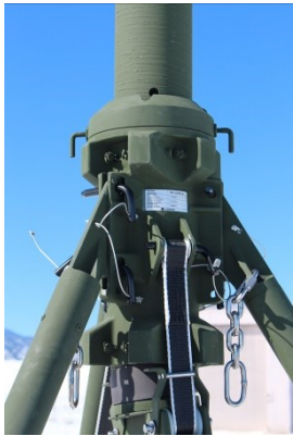
Tripod mast section lifting hoist
