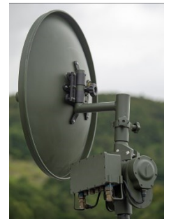
Fully automated payload alignment systems (CAPAS)
