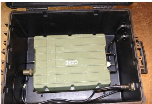
Enhanced Kit - Carrying case used to house HF coupler (coupler not supplied as part of kit)
