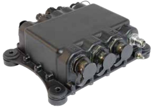
The EZPRR was developed from the basic 256 channel PRR. Data transmission was added to the original voice capability and both voice and data (which can be transmitted simultaneously) are now encrypted. Channel 15 of the EZPRR remains unencrypted to maintain backwards compatibility with the original PRR.
