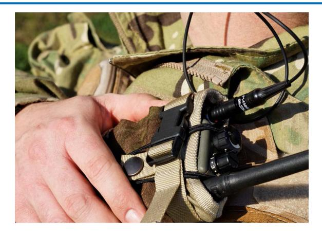
The Enhanced & Encrypted Personal Role Radio (EZPRR) provides AES128 encryption, enabling secure voice and data communications. To meet operational, training and support requirements, Selex ES has developed a modular, ruggedised and lightweight Multi-Fill Unit (MFU) capable of filling up to twelve EZPRR radios in a single operation.
