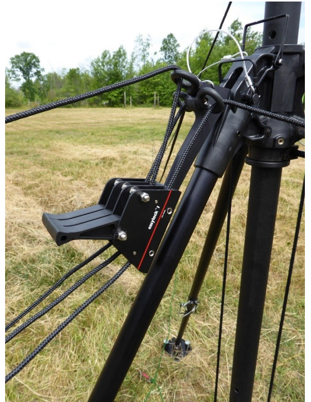
Mast Central Guying System
