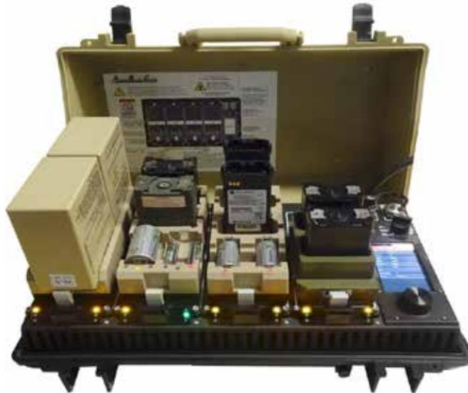
Fast Charging: 8 BB-2590/U batteries charged from 0% to Full in less than 3 Hours
