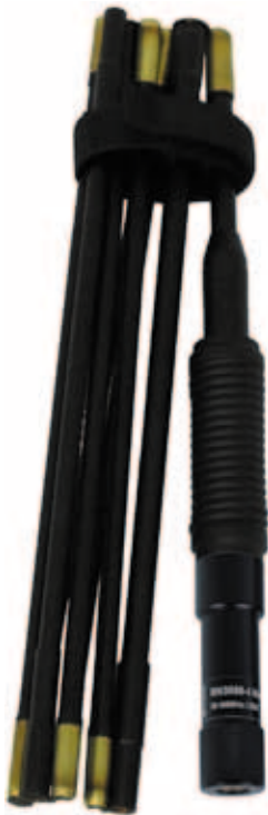
APX28 shown with spring and 25W VHF 30 - 108 MHz antenna matching unit (see overleaf for options)
